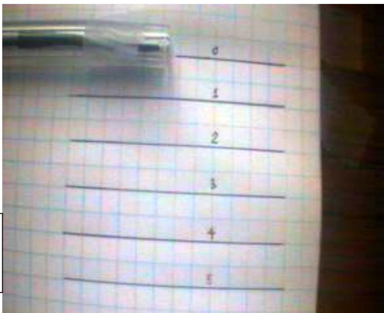
**Fig. 4** Draw regularly-spaced lines at five distances from the sensor tube. ("0" is "no distance" from the sensor, "1" is "one unit of distance from the sensor, etc.)
